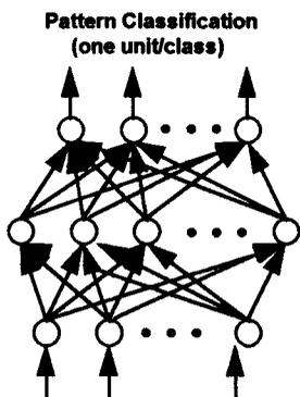
Figure 1 - Multi Layer Perceptron Architecture
