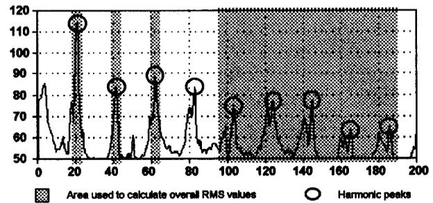
Figure 2 - Spectral feature extraction
