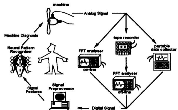
Figure 3 - Neural network vibration signal classification
